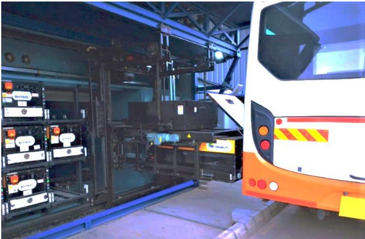
Figure 16. Battery swapping in Ahmedabad, India
